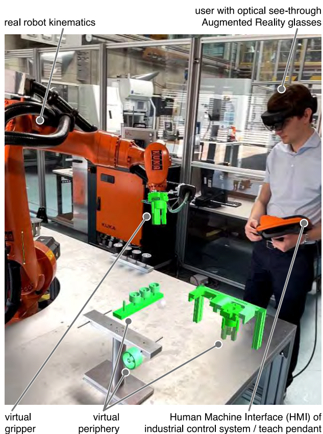
Fig. 2 Exemplary scenario of Mixed-Reality-in-the-Loop Simulation (virtual objects highlighted in green)
