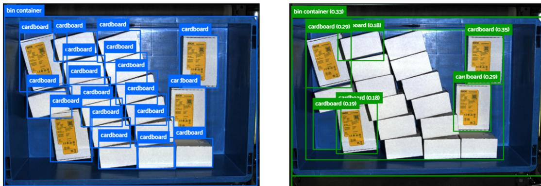
Fig. 3: Ground truth (left) and model predictions of Grounding DINO (right) [5]
